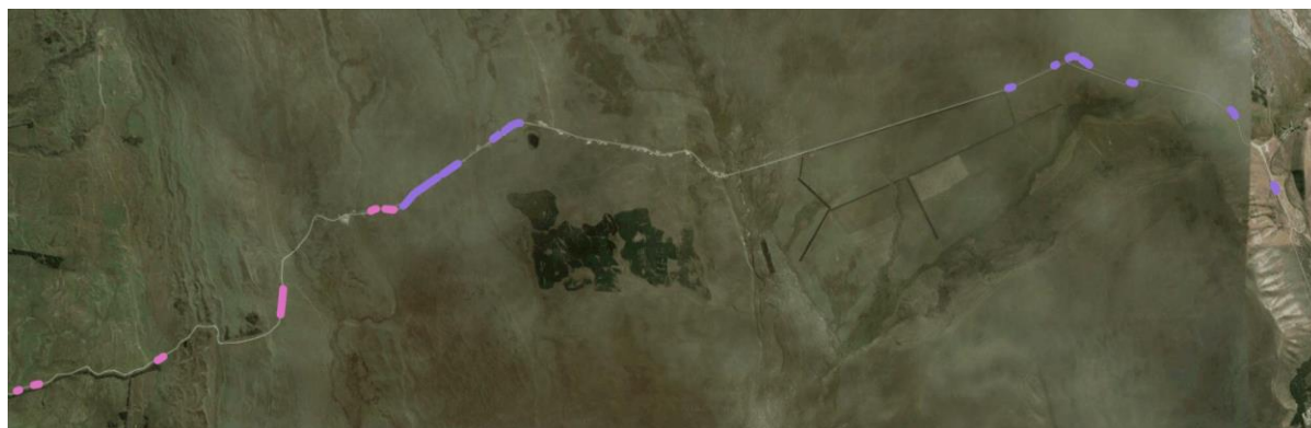
Braemar Road – Frost heave approximately 5km will need a thick wearing course application.
