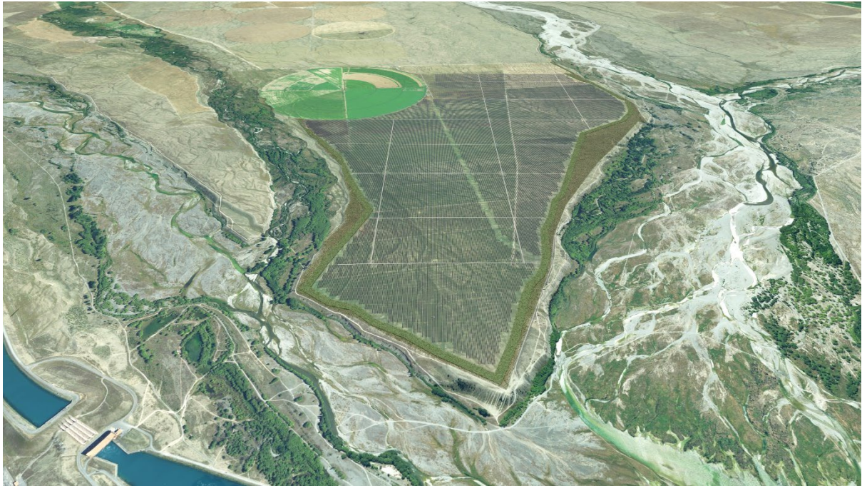
Overview of 3D model showing digital terrain model with solar panel layout and landscaping.
