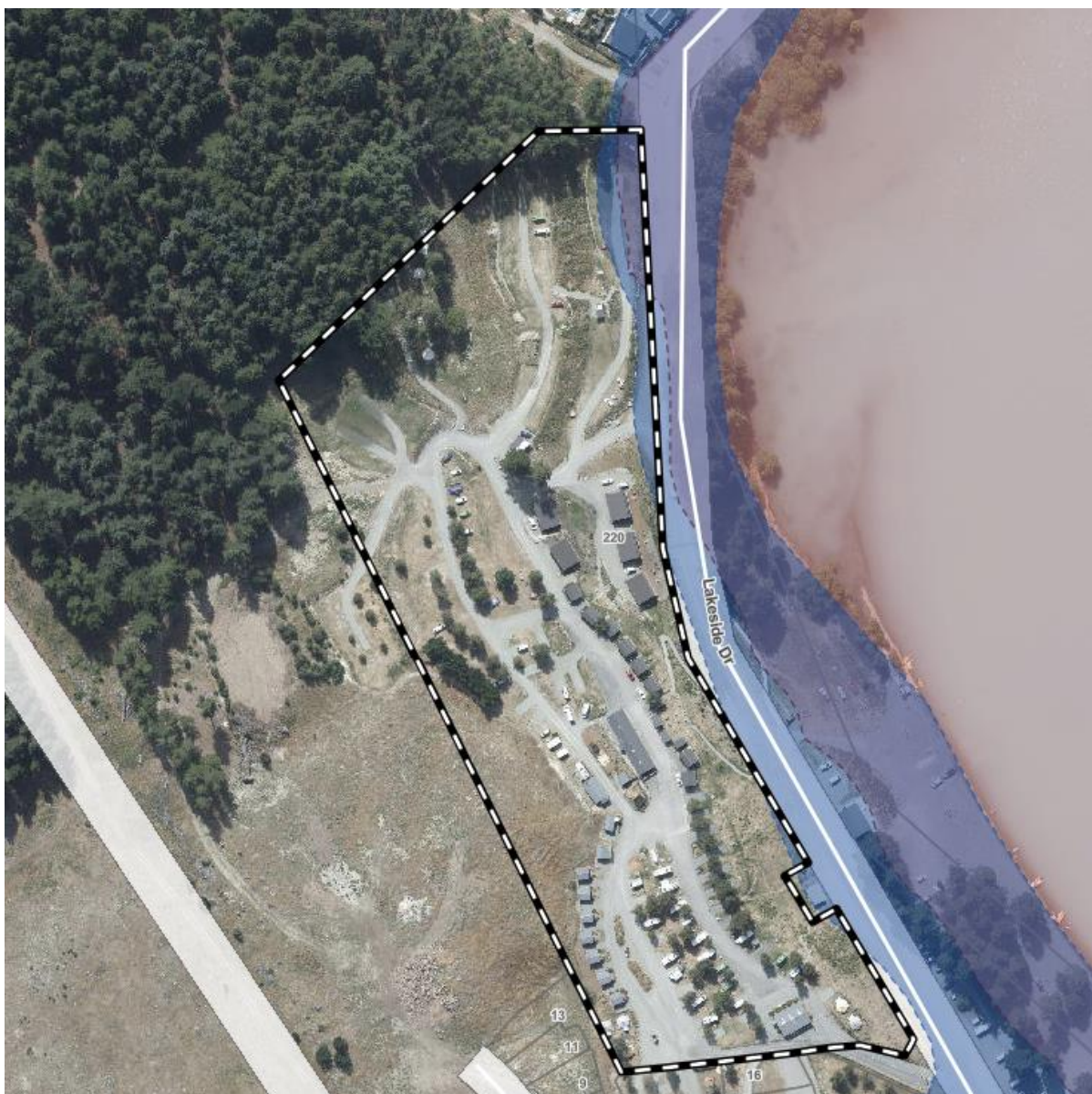
Figure 2: Image showing Flood Hazard Assessment Overlay (red) and Liquefaction Overlay (blue) encroaching eastern edge of submitters site
