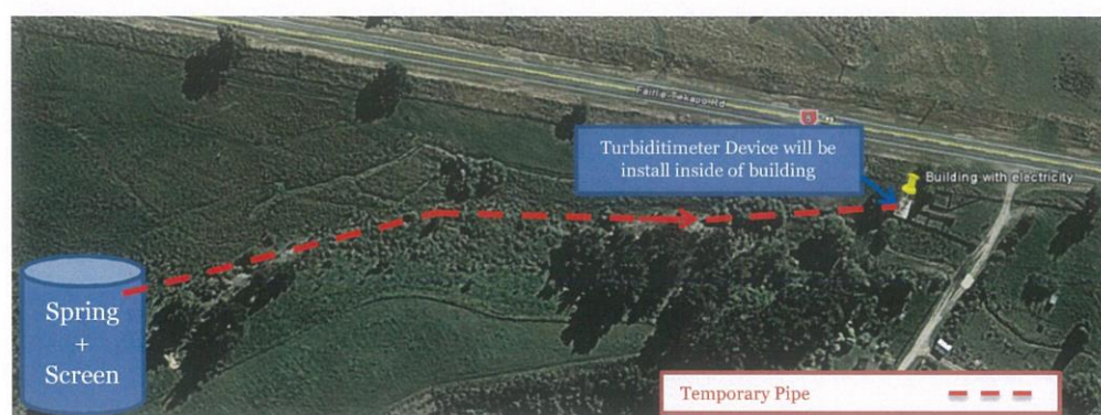
Figure 5. Completely Temporary Pipeline (Option 1) – Outline Route
