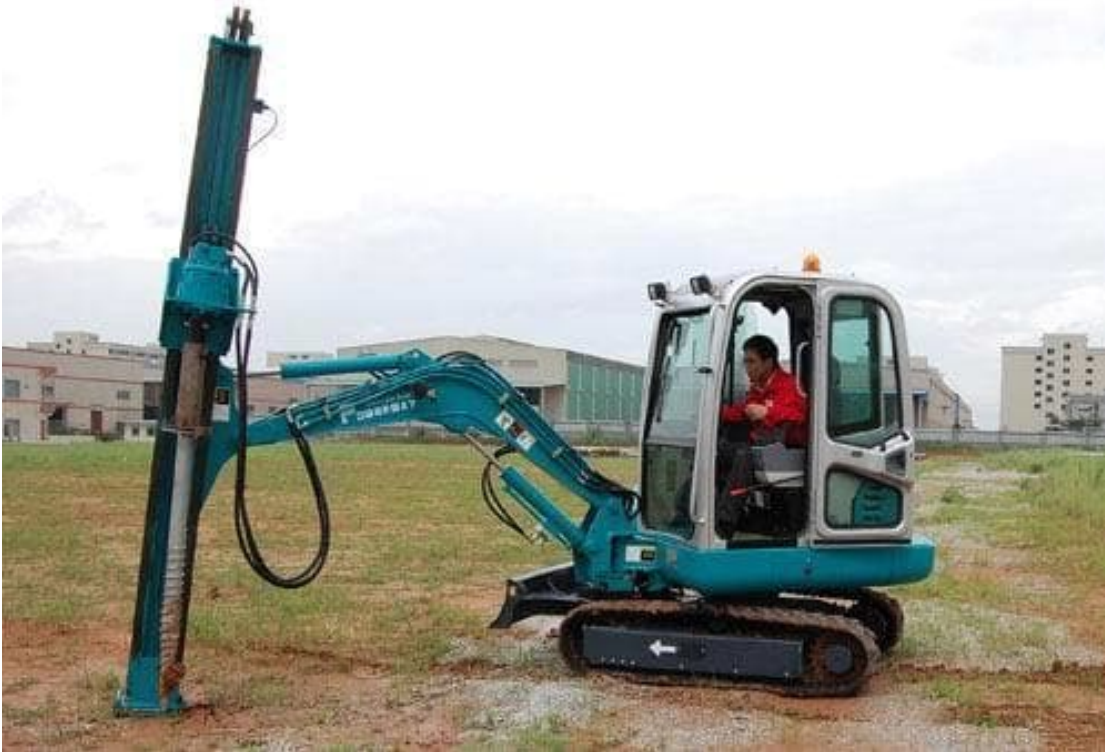
Figure 6. Example of screw pile driving method to be used on site. (Source: FNSF, 2023).
